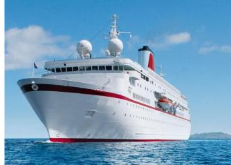
22496GT 8264NT 3460DW ON 5.6M DIM 175.3/155.8 X 23.0M BUILT HDW, GERMANY 05/1998 GL +100 A5 E1 IW MC E1 (HIGHEST ICE CLASS) AUT SOLAS 1997, USCG/USPH 620 PASSENGERS (MAX) 604 BERTHS IN 302 CABINS (224 OUTSIDE CBS)
