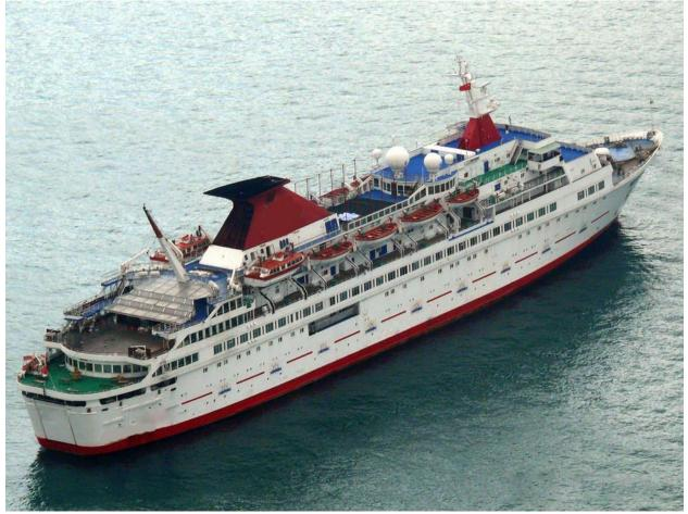
Tonnage: 16,331 GRT 2,251 t DWT Length: 156.27 m (512 ft 8 in) Beam: 22.05 m (72.34 ft) Draught: 5.90 m (19.36 ft) Depth: 16.31 m (53.51 ft) Decks: 9 Ice class: ICE-C Installed power: 2 × Wärtsilä-Pielstick 18PC2V diesels combined 13240 kW Propulsion: Two propellers Speed: 21.50 kn (39.82 km/h) 650 passengers in lower beds, 755 total Location: Hong Kong Price: \$10 million, outright sale only
